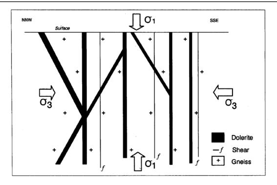
Figure 2: Cross-section showing orientation of metadolerites in the Abbabis Inlier and indicated stress field at the time of their emplacement
