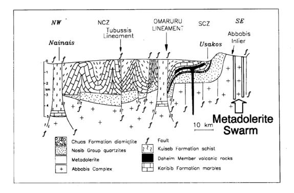
Figure 3: Cross-section through the Central Zone of the Damara Orogen showing basement faults and metadolerite swarm in the underlying mid-Proterozoic basement (after Steven, 1993). Note feeder to Daheim Member volcanic rocks.
